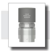
Quick disconnects create a consistent mounting location for portable routes. The receptacle features a triaxial locating notch and ¼ turn engagement onto the stud, ensuring the sensor is oriented in the same position when connected to the stud for every reading.
