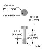
M6x1 Captive Bolt with Socket Head Cap for TREA/TRCA Series Compact Triaxial Accelerometers, 18-8 Stainless Steel, 0.89 in. (22.6 mm) Length
