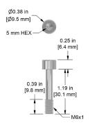
M6x1 Captive Bolt with Socket Head Cap for TXEA/TXFA Series Large Triaxial Sensors, 18-8 Stainless Steel, 1.19 in. (30.23 mm) Length
