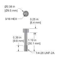
1/4-28 Captive Bolt with Socket Head Cap for TXEA/TXFA Series Large Triaxial Sensors, 18-8 Stainless Steel, 1.19 in. (30.23 mm) Length
