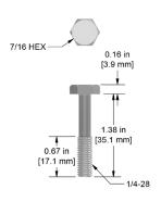
1/4-28 Captive Bolt for CTC TA and VT Sensors, 18-8 Stainless Steel, 1.38 in. (35 mm) Length
