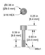
M6x1 Captive Bolt with Socket Head Cap for CTC M/AC119, M/AC115, M/AC230 and M/AC360 Sensors, 18-8 Stainless Steel, 0.93 in. (23 mm) Length
