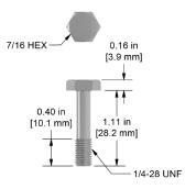
1/4-28 Captive Bolt, for CTC AC194 and AC294 Sensors, 18-8 Stainless Steel, 1.11 in. (28 mm) Length
