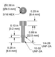
10-32 Adapter Bolt with Socket Head Cap for CTC AC119, AC115, AC230 and AC360 Sensors, 18-8 Stainless Steel, 0.89 in. (22 mm) Length
