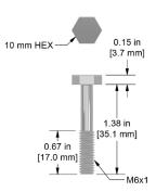
M6x1 Captive Bolt for 500 mV/g, 1000 mV/g Side Exit Sensors, 18-8 Stainless Steel, 1.38 in. (35 mm) Length
