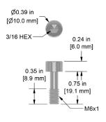
M6x1 Captive Bolt with Socket Head Cap for Miniature Industrial Side Exit Sensors, 18-8 Stainless Steel, 0.75 in. (19 mm) Length
