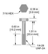
1/4-28 Captive Bolt for Standard Size Side Exit Sensors, 18-8 Stainless Steel, 1.31 in. (33 mm) Length
