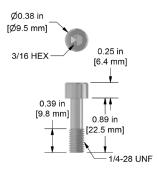
1/4-28 Captive Bolt with Socket Head Cap for CTC AC119, AC115, AC230, and AC360 Sensors, 18-8 Stainless Steel, 0.89 in. (22 mm) Length
