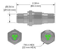
3 Pin MIL to 3 Pin MIL, Bulkhead Feedthrough, 1/2 in. (12.7 mm) NPT, 316L Stainless Steel
