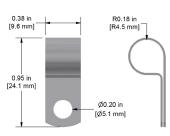
Loop Cable Clamp, 0.25 in. Diameter, 321 Stainless Steel
